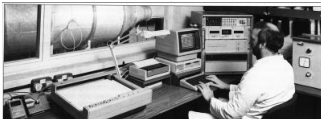
Computer-automated fan test room.
